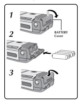
Slide the battery cover (BATTERY) slightly to open.
